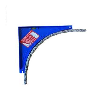
The 8" Radius gauge is a lightning protection tool used to maintain an 8" lightning conductor bend. No lightning conductor should have bends less than 90 degrees with a radius less than 8", this is the industry standard. The radius gauge is helping installers stay up to industry standards and Underwriters Laboratories (UL) is currently using this tool for certification inspections.
