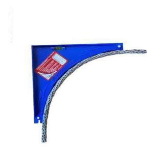
Until now, the 8" radius bend of any lightning conductor has been mostly guess work for installers and inspectors. Kuefler Lightning Protection (KLP) now offers this easy to use 8" radius gauge to you for pocket change. KLP uses this radius tool for every installation, assuring proper bends.
