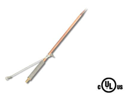
Spring Loaded Air Terminals are used where movable equipment, such as window washing equipment, interferes with Fixed Air Terminals. Also used in mid roof areas, for safety, where Air Terminals could be subject to breakage. Easily retrofit to existing Lightning Protection Systems.
